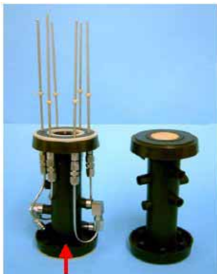
Fully populated core sleeve (Item 21) with "Push-in" type dP ports and \text{\O} 1/8 " process lines aligned axially with the mounted core.
